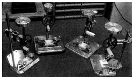
Fig.6 Miniature tapping devices made by students
