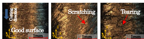
(a) Good surface (b) Scratching (c) Tearing No.13 No.20 No.25
