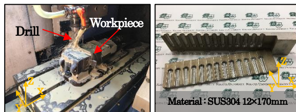
Fig.1 Cutting testing and Workpieces
